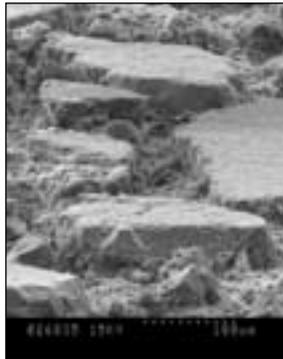
Fig. 5b: Electron micrograph of concrete surface etched with 1M HCl for 15 minutes. The raised areas are siliceous aggregate particles while the depressions are cement paste etched by acid
