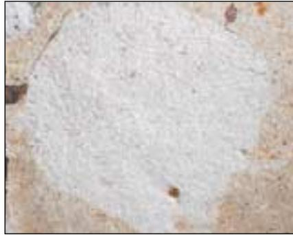
*Fig. 3: Optical micrograph of typical concrete after stripping*
