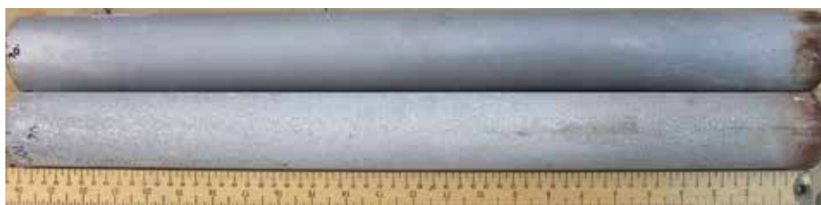
Figure 3: IMM coating (top) and TSA (bottom) on the carbon steel pipes when heated from 95°C (203°F) (left hand side) to 450°C (842°F) (right hand side)
