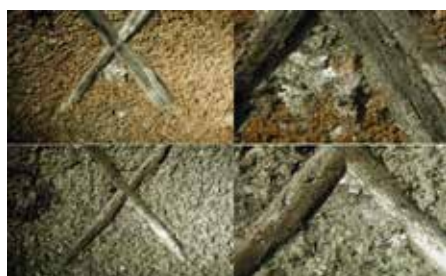
Figure 7: TSA X scribe adhesion. Top row 400°C. Bottom row 100°C. No adhesive disbondment but rust bleed-through visible at 400°C
