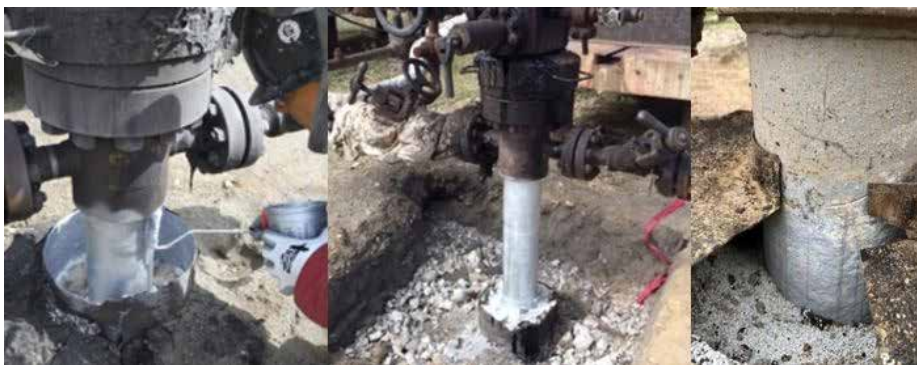
Figure 10: IMM coating immersed on surface casings: day 1 (left), 2.5 years (middle), 10 years (right)
