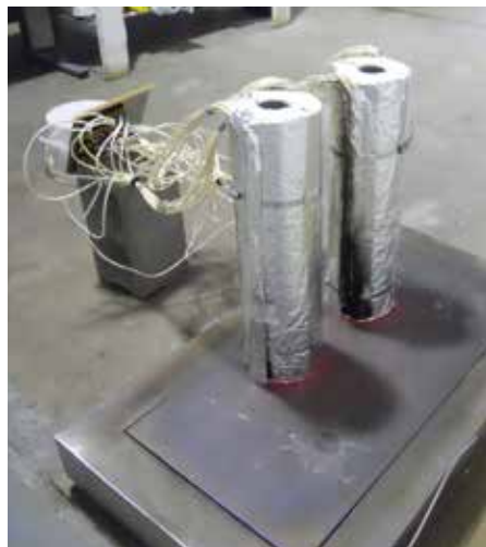
Figure 2: CUI simulated tests of IMM and TSA coated test pipes on a hot plate
