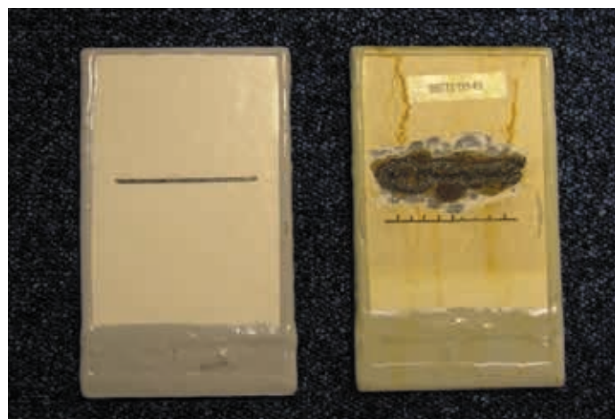
Figure 3 – Typical scribe testing
