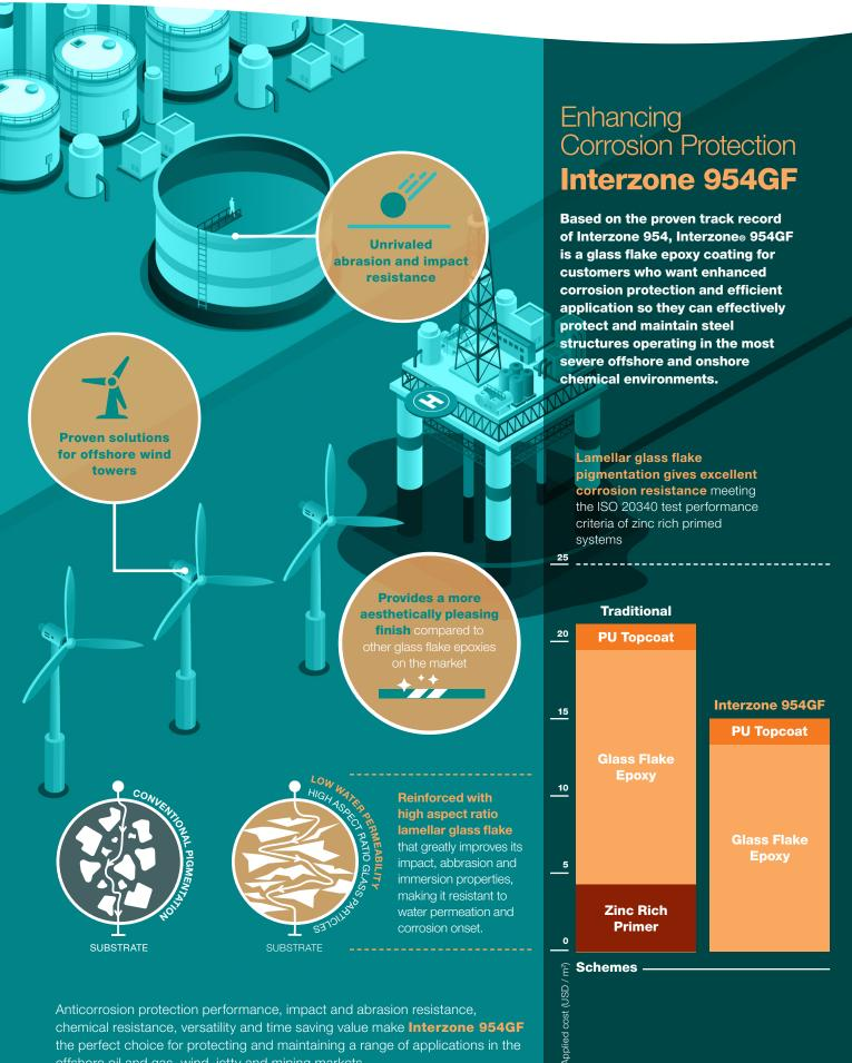
Anticorrosion protection performance, impact and abrasion resistance, chemical resistance, versatility and time saving value make Interzone 954GF the perfect choice for protecting and maintaining a range of applications in the offshore oil and gas, wind, jetty and mining markets.
